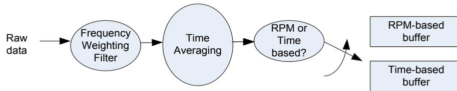
**Figure 148. Time averaged sound level computation.**
