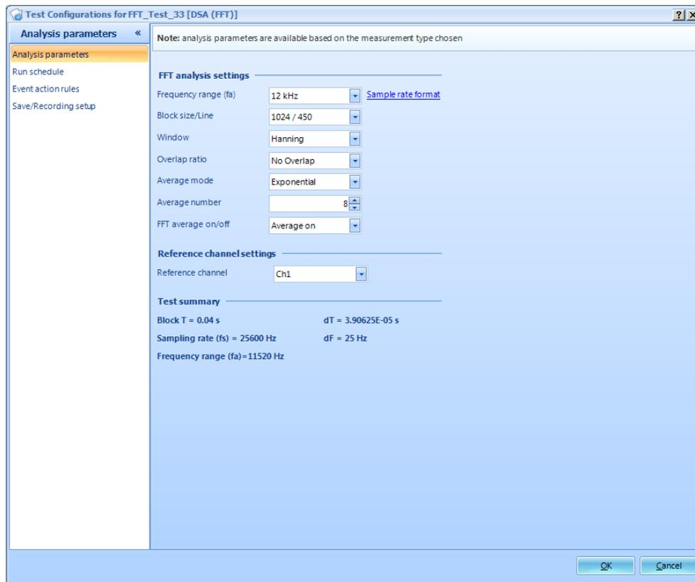
**Figure 130. Analysis Parameters Tab of Test Configuration Window**
