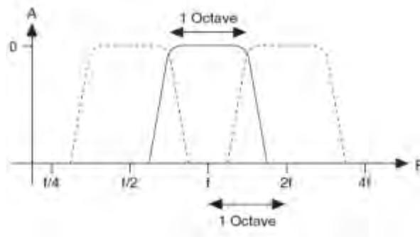
Figure 139. Full octave filter shape.
