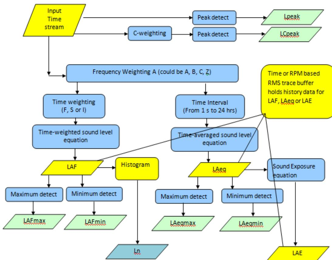
Figure 145. Sound level meter computation diagram.
