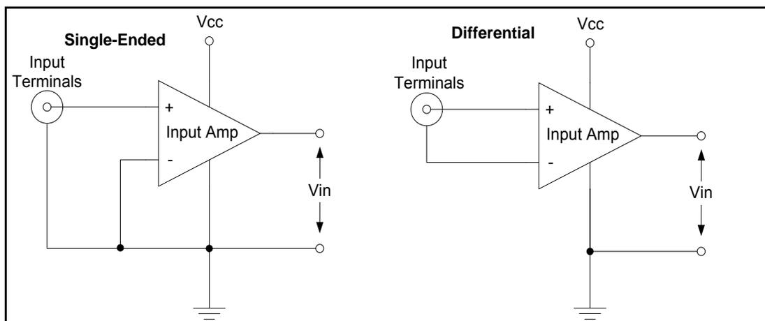
Figure 23: Single-Ended vs. Differential input
