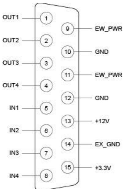
Figure 28. Spider-80X Pin Assignments of DIO Interface Connector
