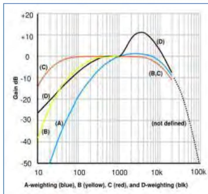
Figure 140. Frequency weighting filter shapes.
