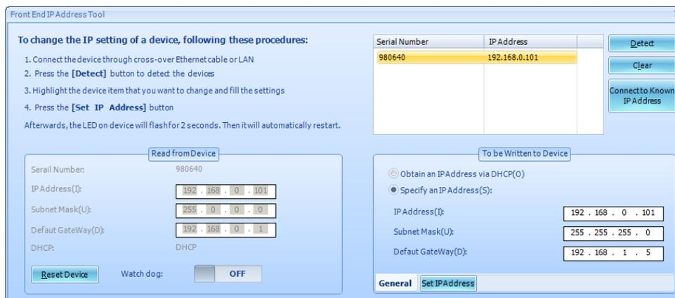
**Figure 2: Set Device IP Address**
