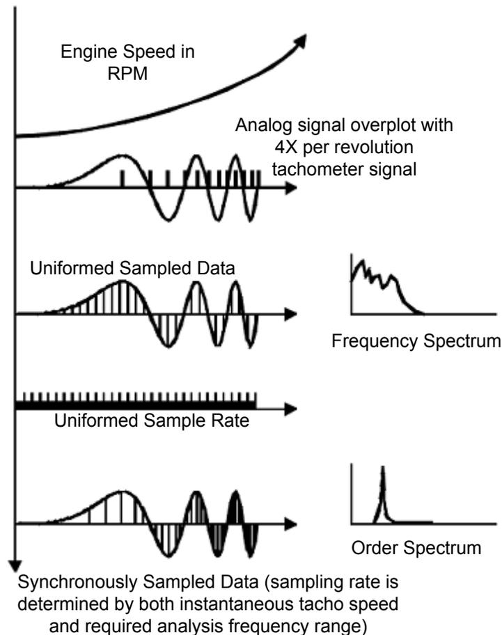
Figure 177: Angular data resampling of a chirp signal
