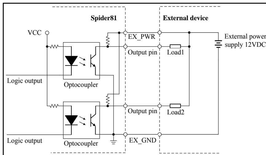
Figure 32. Output Circuit
