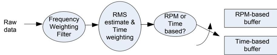
Figure 146. Time weighting sound level computation and storage against RPM or Time
