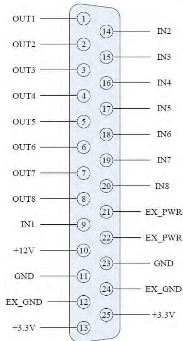
Figure 27: Spider-81 Series Pin Assignments of DIO Interface Connector
