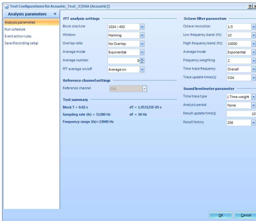
Figure 168. Test Parameters for Acoustic Analysis
