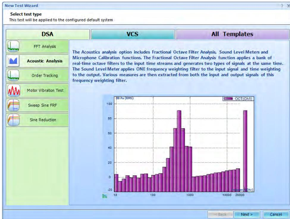
Figure 149: Create a New Acoustic Test
