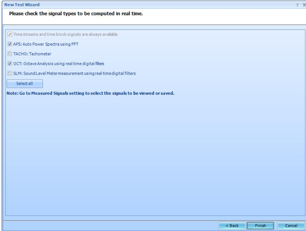
Figure 151. Signal Types in Acoustic Analysis
