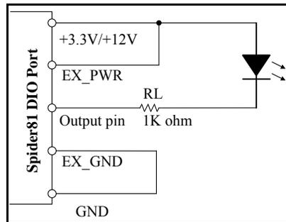
Figure 33. Output Connection to LED
