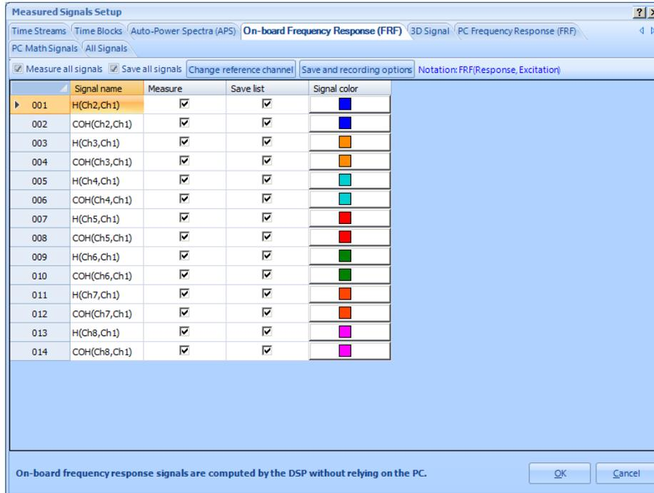
Figure 76. On-board FRF Signals
