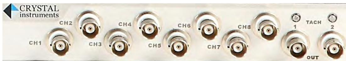
**Figure 21: Spider-80X Input Channels**
