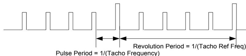
In most tests, the Pulses per Rev will be 1. (Sensing a keyway or other once/turn target is relatively simple.) However, in other situations, such as viewing a toothed flywheel or reference gear, the Pulses per Rev can be as high as hundreds. In general, the higher the Pulse per Rev, the more resolute an order analysis becomes.
