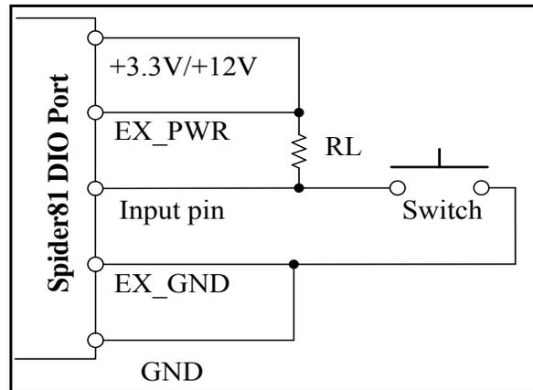
Figure 31. Switch connection to input
