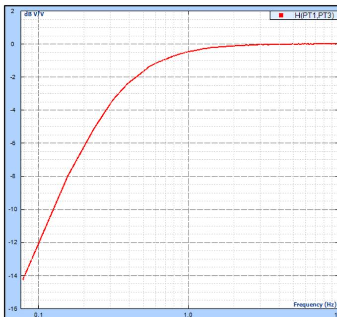
**Figure 24: AC Input Mode High-Pass Filter Shape**
