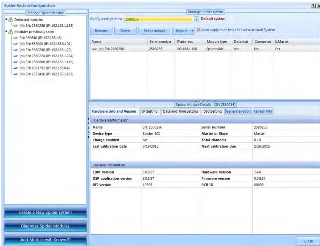
Figure 8: Spider System Configuration
