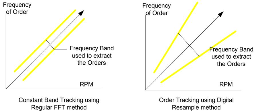
**Figure 178: Comparison of constant band tracking and digital re-sampling method.**
