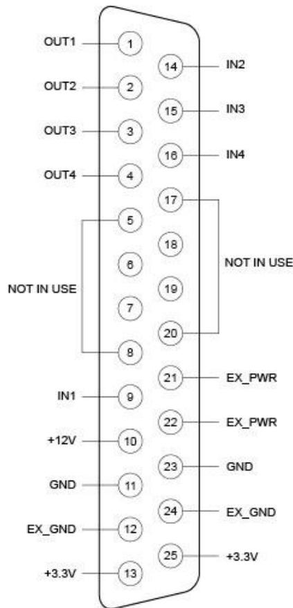
Figure 29. Spider-81B/81C Pin Assignments of DIO Interface Connector
