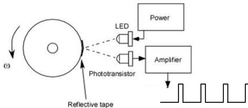
Figure 169. Optical tachometer setup.
