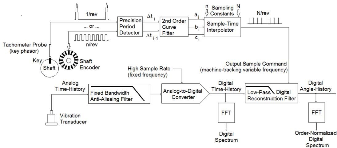
The vibration signal is sampled by an ADC that runs at a *constant* 102.4 kHz sample rate and is protected by a *fixed-frequency* anti-aliasing filter. The bandwidth of this filter, **F<sub>span</sub>**, is selected such that ...
