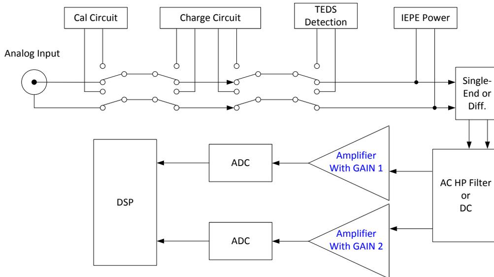
Figure 22: Typical Input Block Diagram (Spider-80x and Spider-81)
